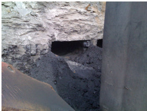
Auger drill holes at Mill Creek
