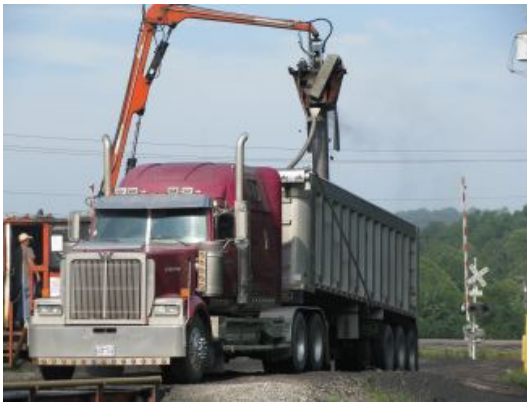
Coal sampling at wharf
